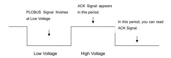
At the first cycle High Voltage after PLCBUS Signal is received, ACK Signal begins feedback. You can estimate whether there is ACK Feedback Signal by reading R\_ACK\_PULSE bit from RX\_TX\_SWITCH Register.
