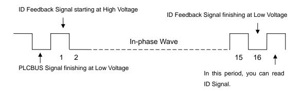
At the first cycle High Voltage after PLCBUS Signal is received, ID Signal begins feedback. After 16 and a half-cycle, it will finish in Low Voltage Cycle. You can estimate whether ID Signal has been received finishing by reading R\_ID\_PULSE bit from RX\_TX\_SWITCH Register. If received finishing, reading ID Signal by Register R-DATA1、R-DATA2:
